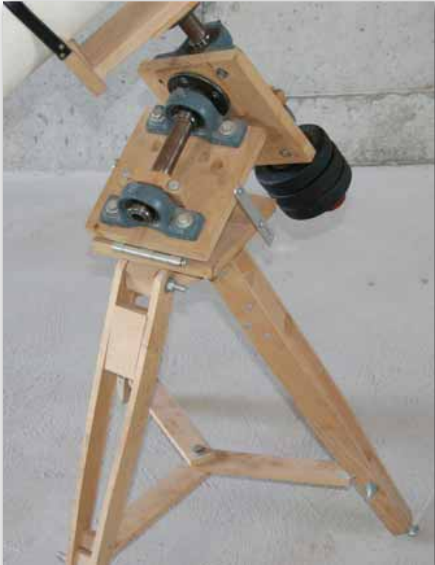
The image above shows several home-made components including a hose clamp and v-block finderscope mount. No finder or eyepieces came with the telescope but there were a lot of other nice surprises.
