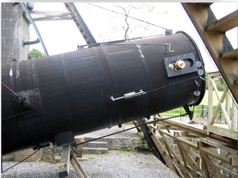
Right: The Leviathan of Parsonstown as it appeared in 2011. One of the two speculum mirrors (left) of 5 that were cast is on display at the Science Museum in London England. The telescope at Birr Castle has been rebuilt and an aluminum mirror (not glass) was installed in the tube for viewing in 1999. The telescope is in use for star tours today.
