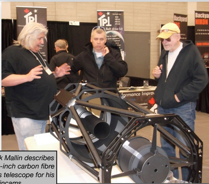
Hercules scope business end -four focuser ports and a motorized secondary!
