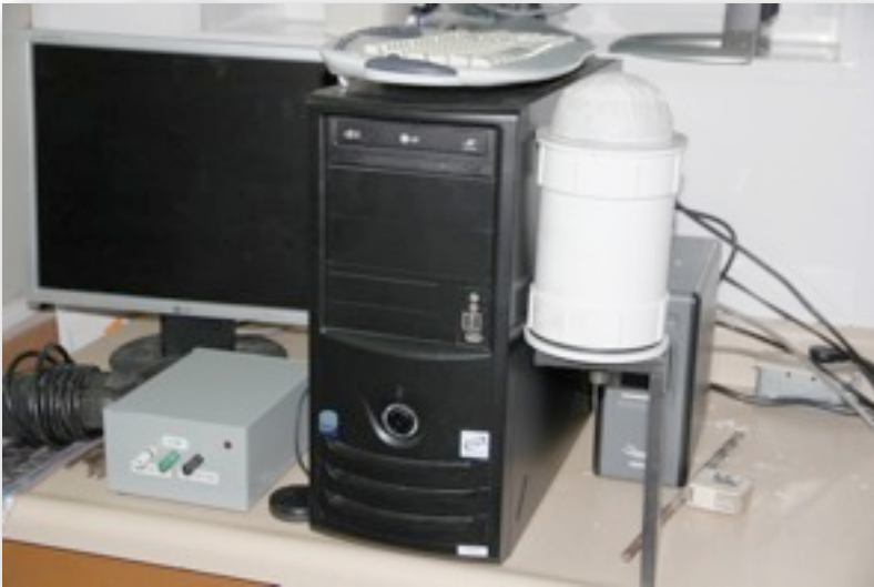
Zbyg was very proud of the smaller version of the camera shown here (4" diam by 10" long). Yes, the camera container is plumbing pipe! The transparent acrylic dome is still covered with protective tape.
