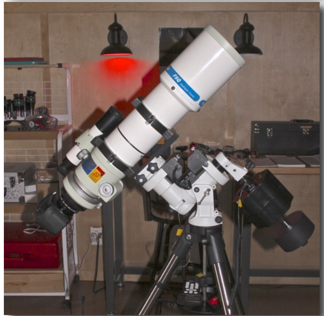
Above: Light weight, wide-field, imaging platform, TAK FSQ 106, iOptron ZEQ 25 and Canon 60Da. The large black counterweight is actually a rechargeable battery. Notice the Unique “Z” Configuration of mount head. Cunningham Photo
