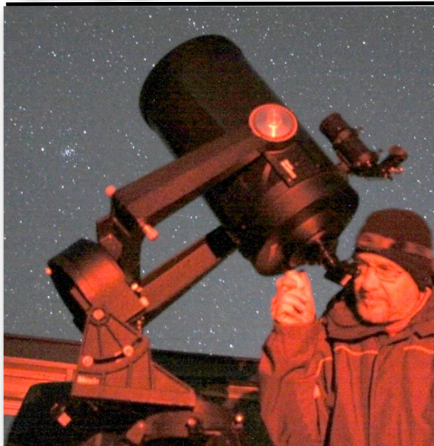
This 10-inch Meade SCT donated by Jim and Dora Bishop. On a new AZ-EQ6 mount it has become the workhorse scope at the Fox Observatory.
