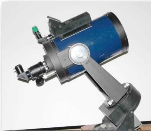
The first scope obtained by BCAS - a Meade 8-inch SCT. Dr. Herb Coleman also gave a 2-m dome and accessories. A additional rack focuser is attached to the diagonal holder to do the coarse focus, and then fine focus with the traditional focus knob.
